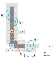
Figure 2. The tracklet model described by its position (x,y) and four reference object landmarks (blue) initiallized from the blob contour (light gray). The ellipses depict the landmark covariances. Although the example shows only one tracklet assigned to one grid cell (red), we initialize new tracklets with random landmark in every newly observed cell (a measurement cell that was not associated yet to any existing tracklets).
