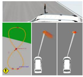
Figure 7. Top: a simulated scenario containing one pedestrian moving in an eight-shape trajectory. Bottom-left: the trajectory of the moving pedestrian. Bottom-center: the extracted dynamic tracklets represented by speed vectors. Bottom-right: the estimated dynamic grid with colored cells. Both tracklets and estimated grid cells are two alternative ways to represent the same target and are colored based on motion direction and magnitude.
